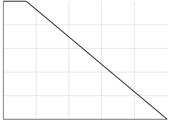
Fig.8 Maximum Power Dissipation Derating vs. Case Temperature
